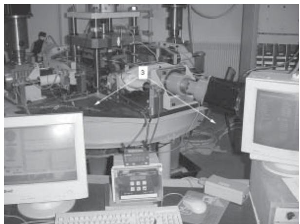
Figure 4. Testing machines and data acquisition systems, a) Triaxial machine in 3S ; b) Triaxial machine in LMR ; c) Direct shear machine in 3S (1- axial jack, 2- confining pressure system, 3- data acquisition system, 4-axial brushless servo-motor, 5- shearing brushless servo-motor).
