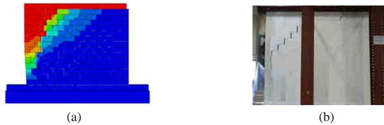
Figure 3. Deformation and crack pattern of the retrofitted masonry walls subjected to lateral load: a) Numerical; b) Experimental
