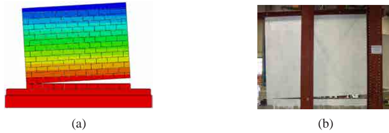
Figure 2. Deformation and crack pattern of the unreinforced masonry walls subjected to lateral load: a) Numerical; b) Experimental
