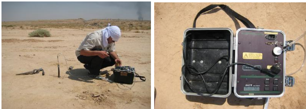
Figure 2. Measurement of Gas Radon in the field
