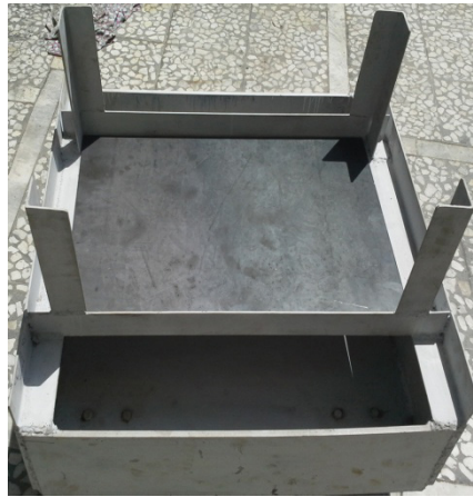
Figure 2. One degree of freedom model for testing on shake table
