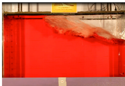
Figure 1. Tank model excited by harmonic oscillation
