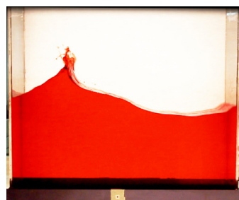
Figure 1. Rectangular storage tank under seismic excitation
