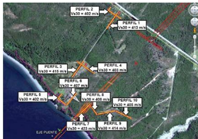
Figure 1. Spatial Distribution of the Seismic Surveys Performed and Vs30 Values, North Side
