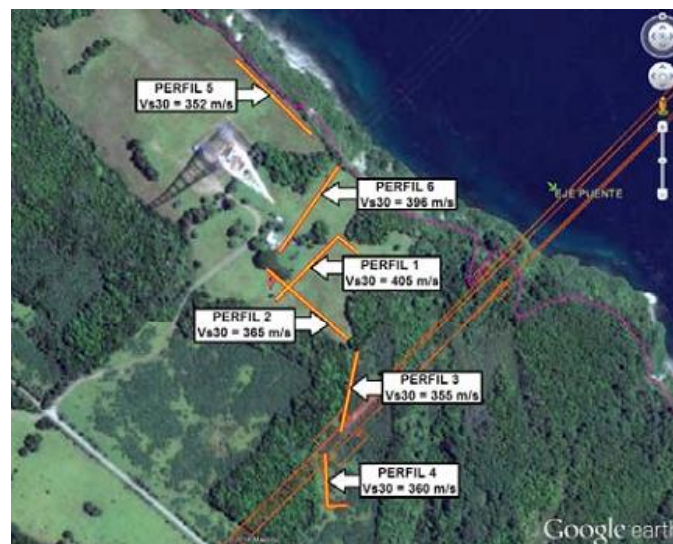
Figure 2. Spatial Distribution of the Seismic Surveys Performed and Vs30 Values, South Side
