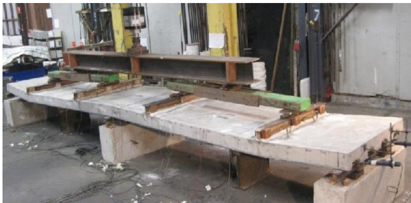
Figure 4. Final deflected shape of slab S1
