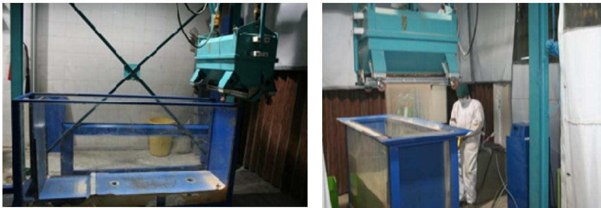
Figure 2. The 1-g model tests apparatus (left) and the pluviation technique with an electric sand rainer (right)
