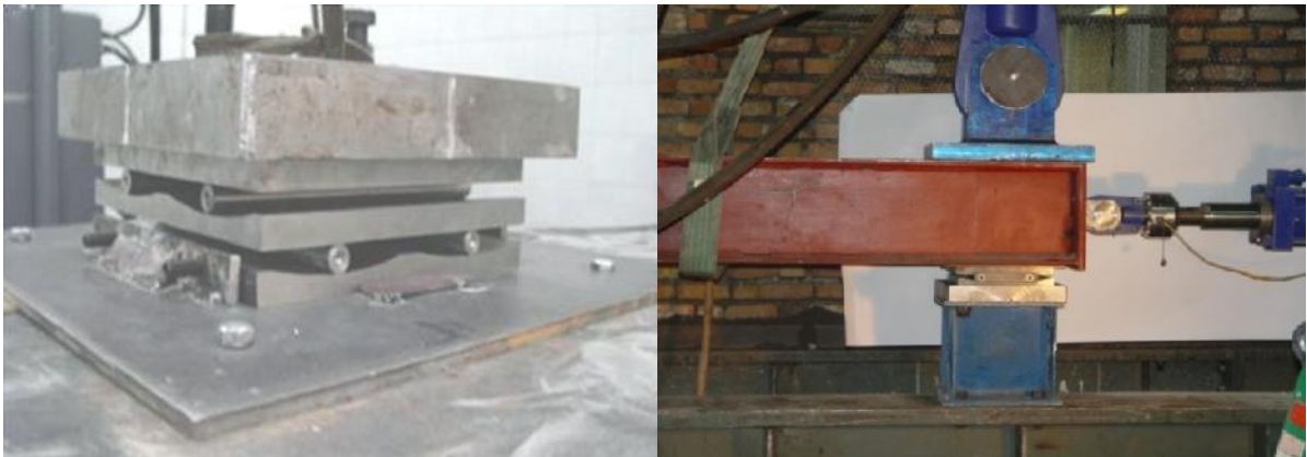
Figure 1. The proposed OPRCB base isolation system installed on shake table (left) and a pair of them under constant vertical and cyclic lateral loading (right) (Hosseini and Soroor, 2011)
