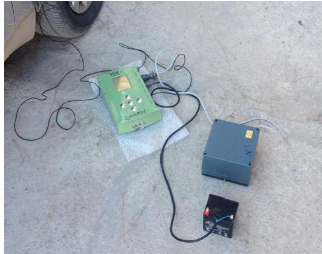
Figure 2. The 3-components seismometers and PDER data logger
