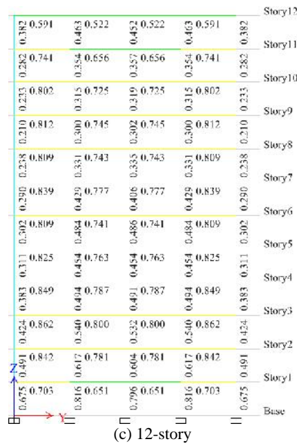
Figure 3. Demand capacity ratio for structural elements
