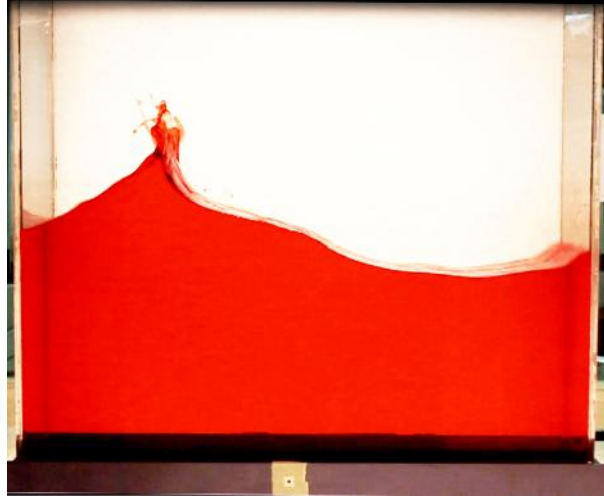
Figure 3. Rectangular storage tank under seismic excitation
