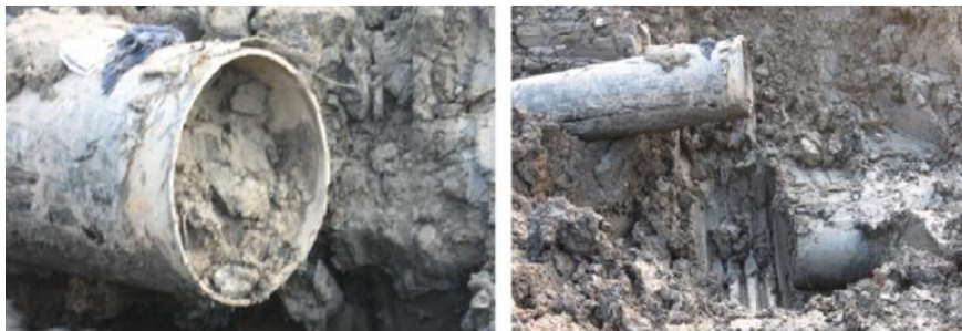
Figure.3. Captions near the fracture location of accident pipeline. [Zheng J.Y., et al. (2012)]
