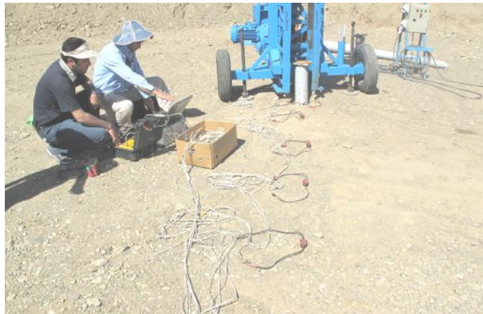
Figure 5. Geophones arrays in ground vibration tests
