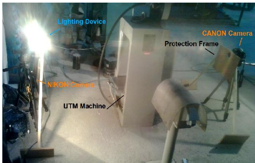
Figure 2. A schematic view of loading setup
